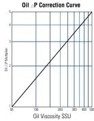
Performance Curves are based on 50 SSU oil entering the cooler  $50^{\circ}$ F higher than the ambient air temperature used for cooling. This is referred to as a  $50^{\circ}$ F E.T.D.
